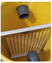
Filtration with the perforated stainless steel filter sieve
