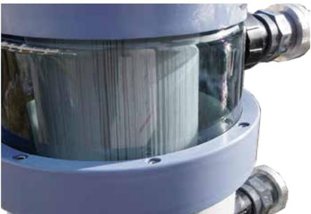
The paper filter cartridge gets dirty very quickly, depending on the type of dirt. This requires frequent backwashing.
