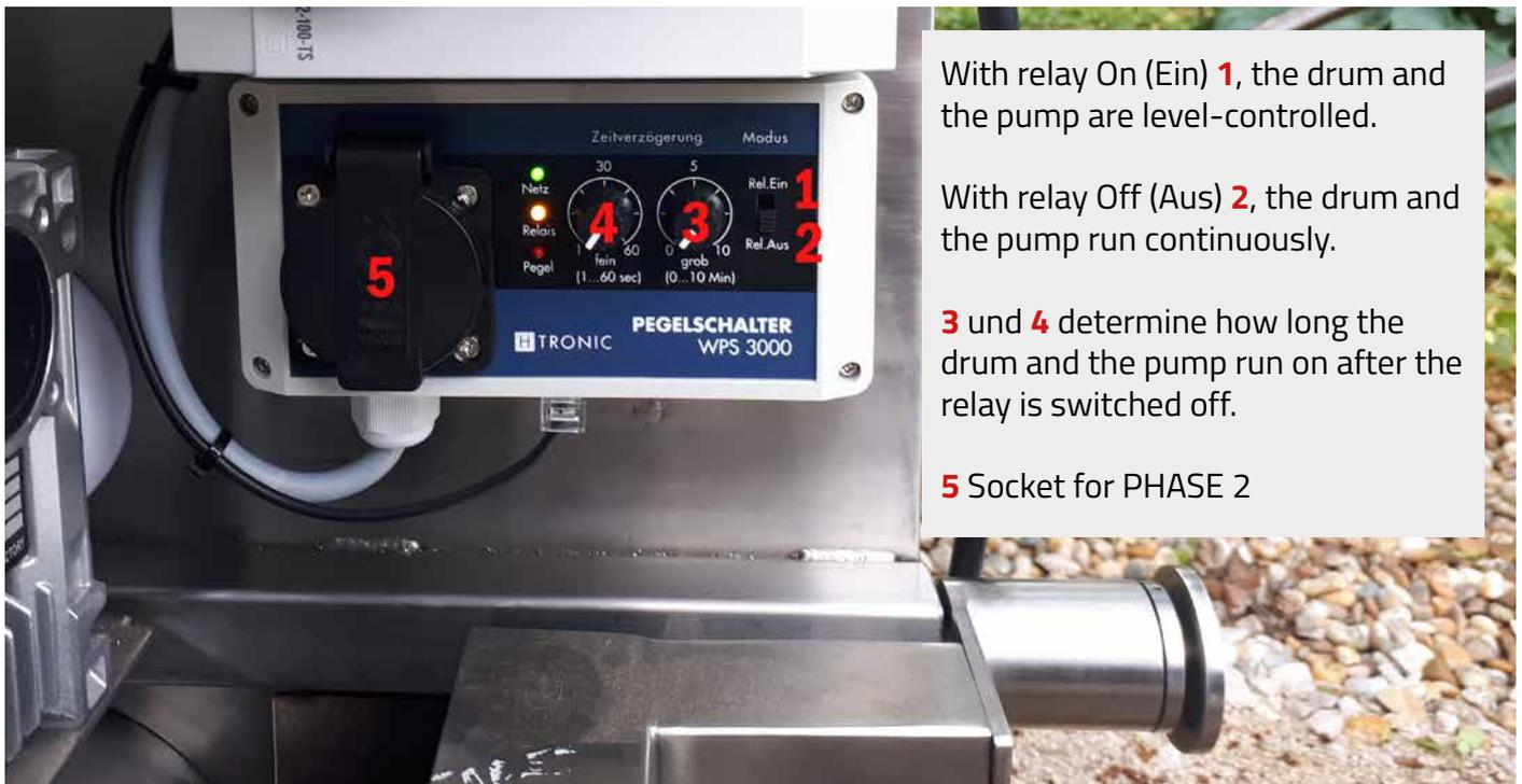
With relay On (Ein) **1**, the drum and the pump are level-controlled.
