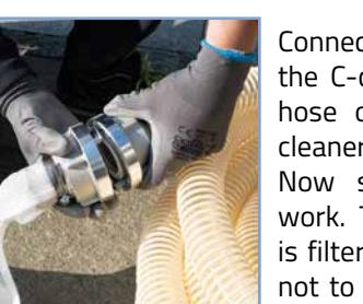
Connect the fine filter bag to the C-coupling of the drain hose of the pond suction cleaner. Now start the extraction work. The sucked-in water is filtered slowly. Be careful not to overfill the fine filter bag, otherwise it could burst.
