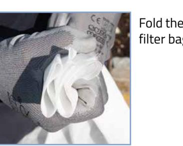
Fold the open end of the fine filter bag like a bellows.
