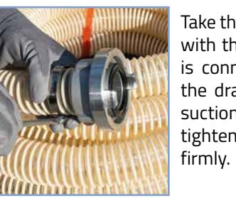
Take the C-coupling enclosed with the fine filter bag. This is connected to the end of the drain hose of the pond suction cleaner. To do this, tighten the hose clamp firmly.
