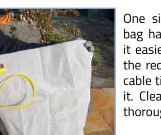
One side of the fine filter bag has a opening, making it easier to be cleaned. Use the red lever on the special cable tie to unlock and open it. Clean the fine filter bag thoroughly.
