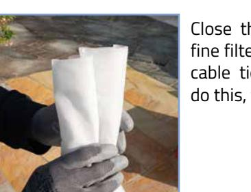
Close the open end of the fine filter bag again with the cable tie after cleaning. To do this, follow steps 6 to 9.
