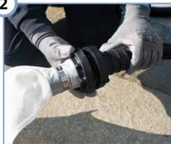
Connect the fine filter bag to the C-coupling of the drain hose of the pond suction cleaner. Now start the extraction work. The sucked-in water is filtered slowly. Be careful not to overfill the fine filter bag, otherwise it could burst.
