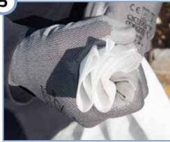
Fold the open end of the fine filter bag like a bellows.
