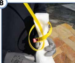
Pass the end of the cable tie through the loop formed during folding to secure it.
